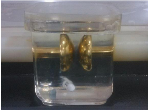
Fig. 3. Brass spherical electrodes of the automatic 50 Hz electrical breakdown tester.
